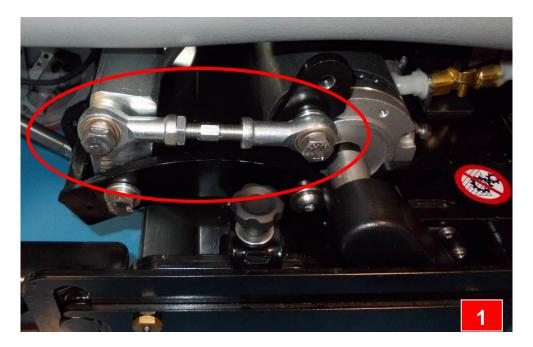
Is possible regulate the brushes pressure by the parts marked in the photo (part.2 figure 4.19): screwing the nut the pressure decreases, unscrewing the pressure increases.
