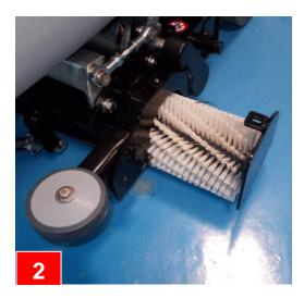
To clean the waste collection tray you have to remove it from his position, you have to pull the handle placed on the right side of machine. (part.3 figure 4.18).
