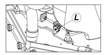
In a properly adjusted squeegee, the front blade should lightly touch the floor and be almost perpendicular to it.
