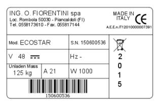
The identification of the machine can be verified by means of a self-adhesive plate on its outer surface displaying indelible details related to "CE" marking.
