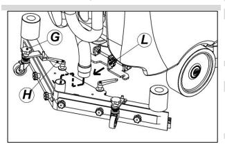
These must therefore be loosened in order to remove the squeegee or insert it in the support arm.
