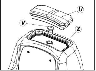
Lift the cover (U). Clean and wash the inside of the tank (5) and the cover with clean water.
