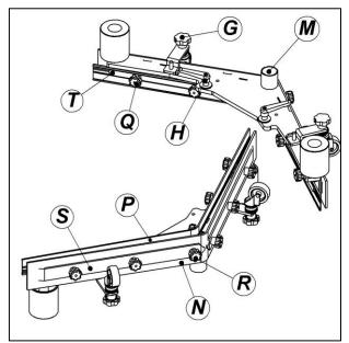
Check that the front rubber (P) and rear rubber (N) are both intact, with no cuts and lacerations, otherwise replace them as indicated below.
