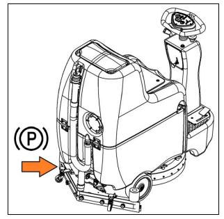
Pull the red lever to disengage the drive. This allows the machine to move freely.
