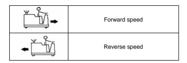
By means of the forward/reverse pedal the operator can move the machine. The operator has to put the foot onto the pedal and press it with the heel to move forward or with the top of the foot to move the machine backward.
