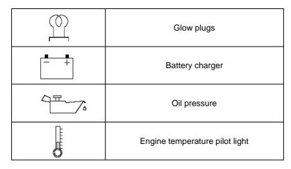
Insert the key into the dashboard and turn it once clockwise. Wait until the glow plugs pilot light (picture nr. 2 position 7) switches off and turn again the key clockwise in order to start the engine.
