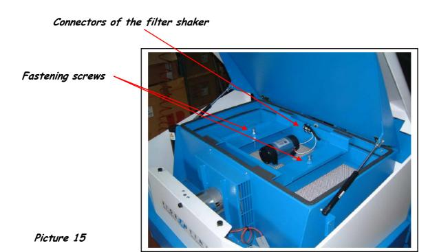
Thanks to the vibrations of the filter shaker engine, the dust falls down from the filters into the waste tank. If it is necessary, remove and replace the filter shaker engine.
