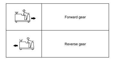
By means of the forward/reverse pedal the operator can move the machine. The operator has to put the foot onto the pedal and press it with the heel to move forward or with the top of the foot to move the machine backward.
